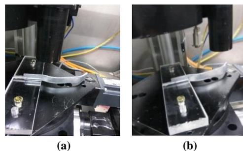
Fig. 9: (a) Initial position of confocal while measuring bending radius (b) Final position of confocal while measuring bending radius
