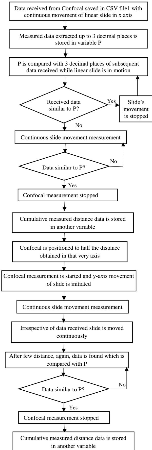
Fig 11: Flowchart for Calculation of bent radius
