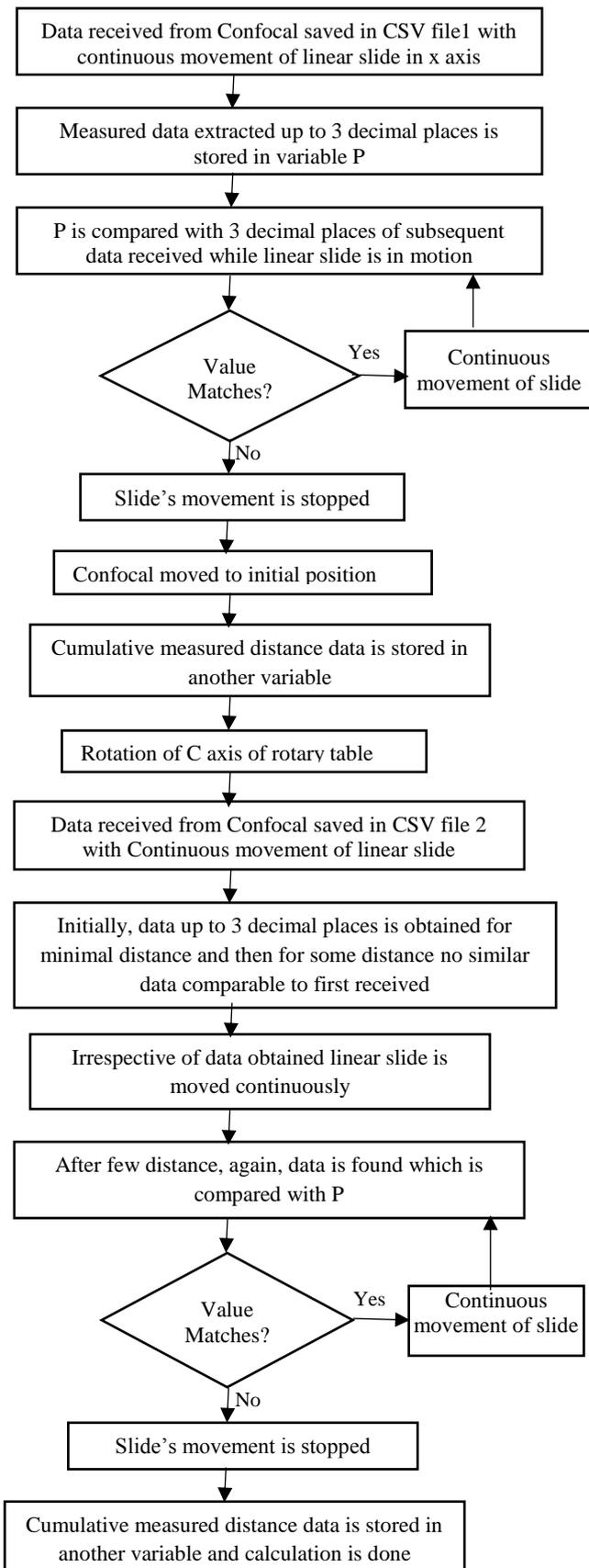
Fig 7: Flowchart of C# program for automated measurement of bending angle
