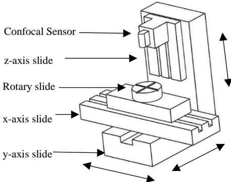
Fig. 2: Schematic diagram of Confocal mounted on z-axis slide with all 4-axis shown.
