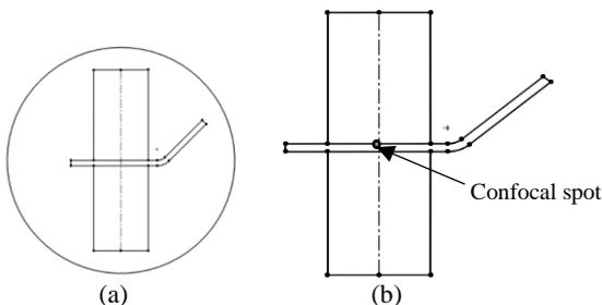
Fig. 4: Schematic diagram of (a) Plate arrangement shown at rotary table (b) Confocal spot shown at center of fixture
